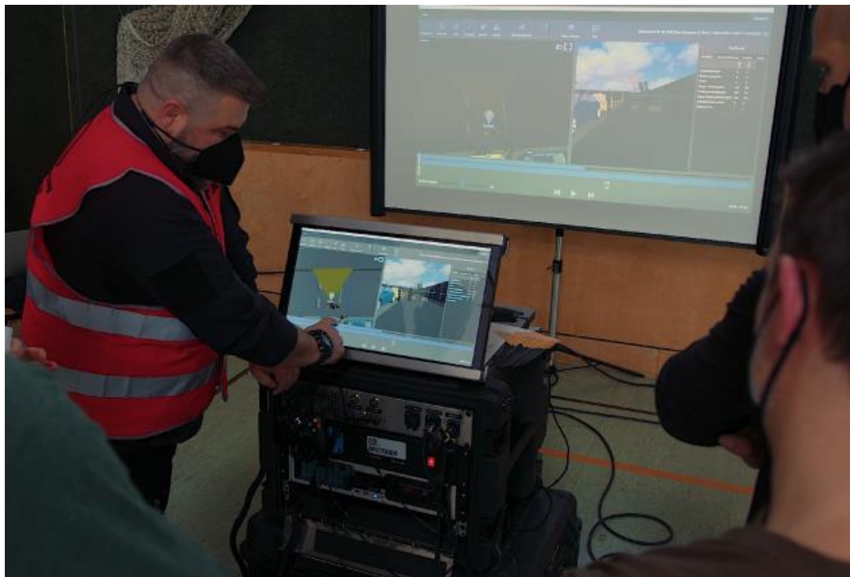
Figure 22: AAR at the trainer station (touch screen for the trainer and big screen for viewers)
