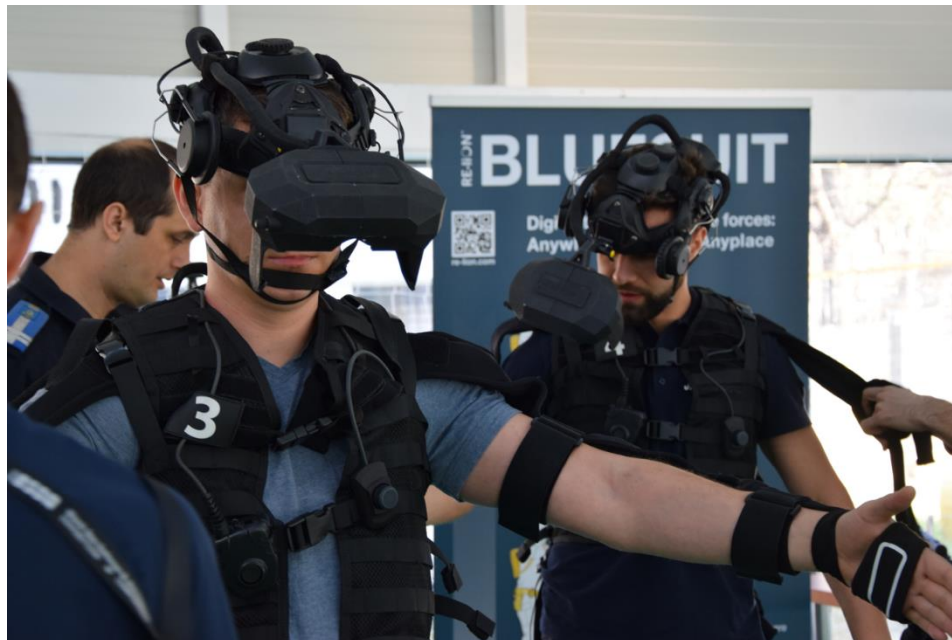
Figure 10: SHOTPROS VR solution – body tracking sensors in Smart Vest (e.g. white square on palm)
